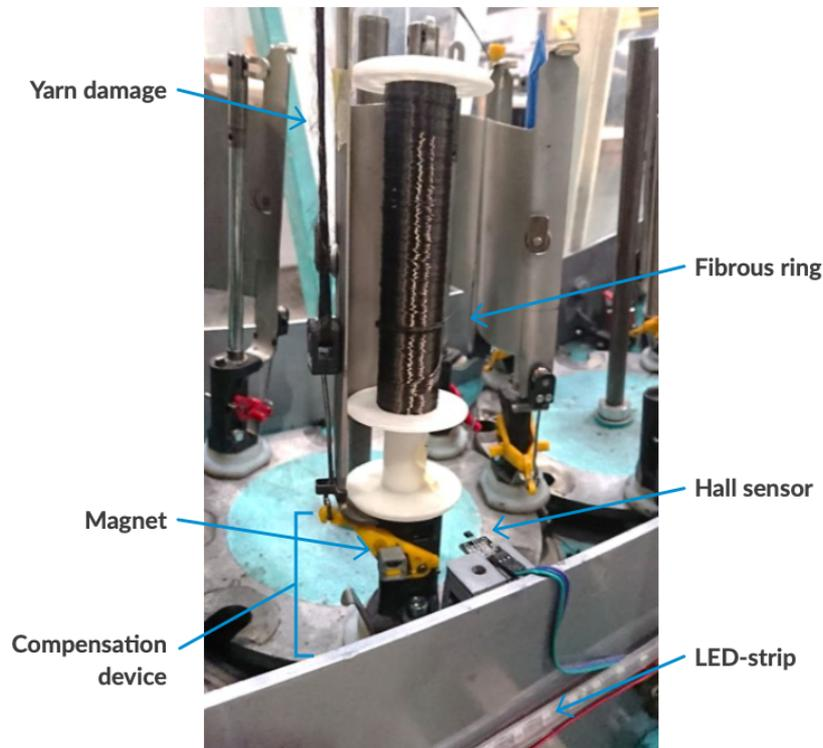
Fibrous ring (accumulation of broken filaments) as an example of an unwinding-related irregularity that impedes the yarn from unwinding properly from the bobbin causing considerable yarn damage, magnet attached to lever of compensation device, stationary hall sensor next to track of bobbin carriers and LED-strip displaying the position of the error cause.
