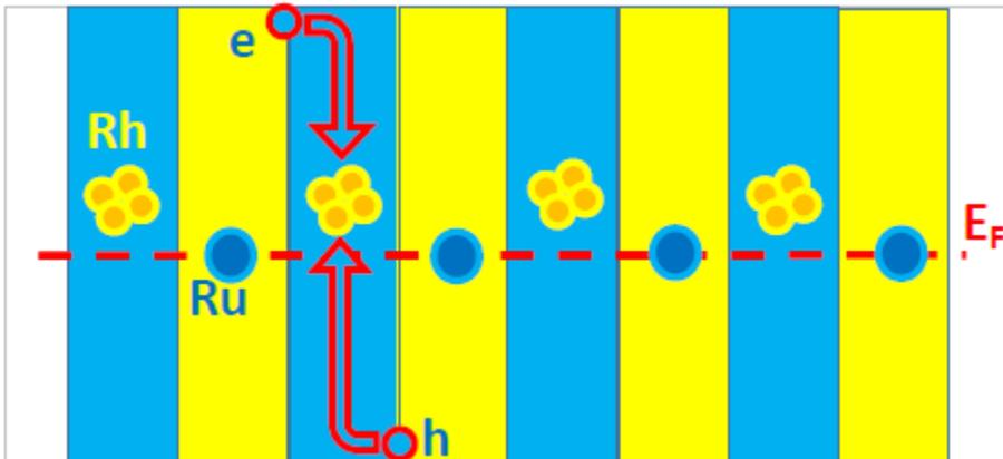
Illustration of the functionality of the dually-doped short-period-superlattice photoconductor. Ru-doped layers pin the Fermi level  $E_F$  in the middle of the semiconductor band-gap, resulting in a high electrical resistance of the material. Rh clusters in the alternating layers provide the ultra-fast electron-hole recombination centers, resulting into ultra-short recombination times.
