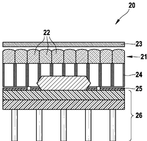
Figure 1: Optical detector with micro lenses
