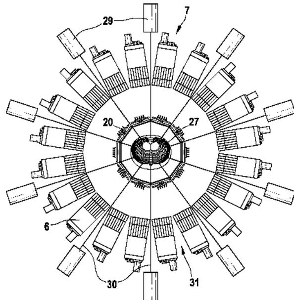
Figure 2: Transaxial view of a dual-modality imaging system
