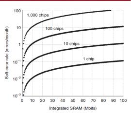
Monthly system soft error rate as a function of the number of chips in the system and the amount of embedded SRAM per chip.
