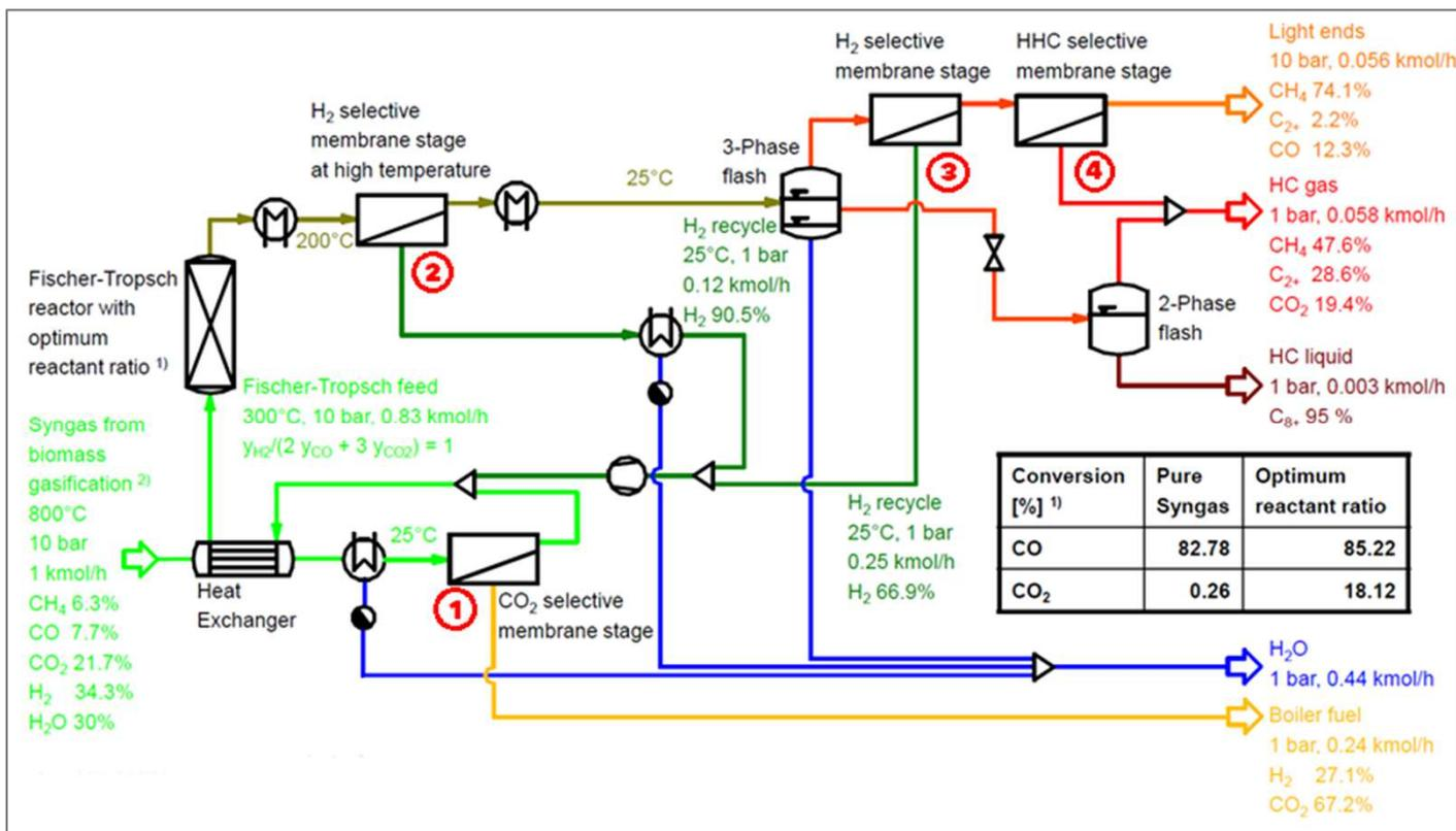
Scheme of the system including the membrane positions, identified in red circles (process design example).
