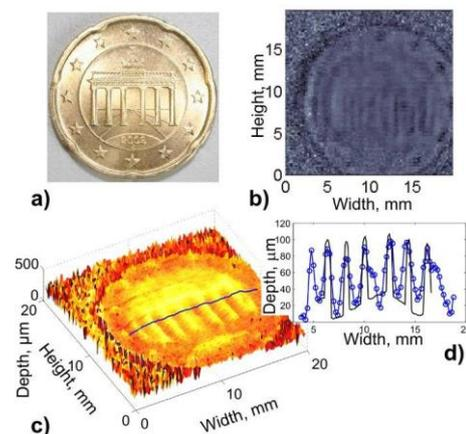
*Elevation profile of a 20 cent Euro coin recorded with a CMOS-push broom scanner.*
