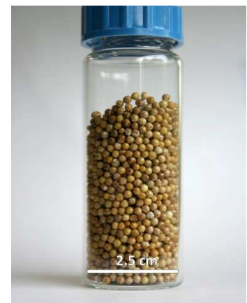
Final composite material with beads in the size of 2 mm. Different salts can be incorporated depending on the required application conditions.
